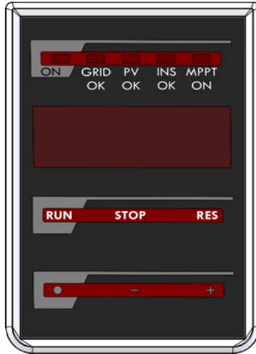
Figure 32 – Remote keypad for PV application
