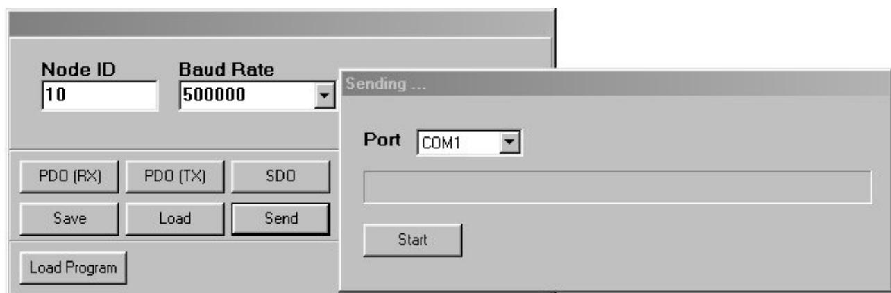
Configurations can be saved and loaded from the PC hard disk through commands “Save” and “Load”.
