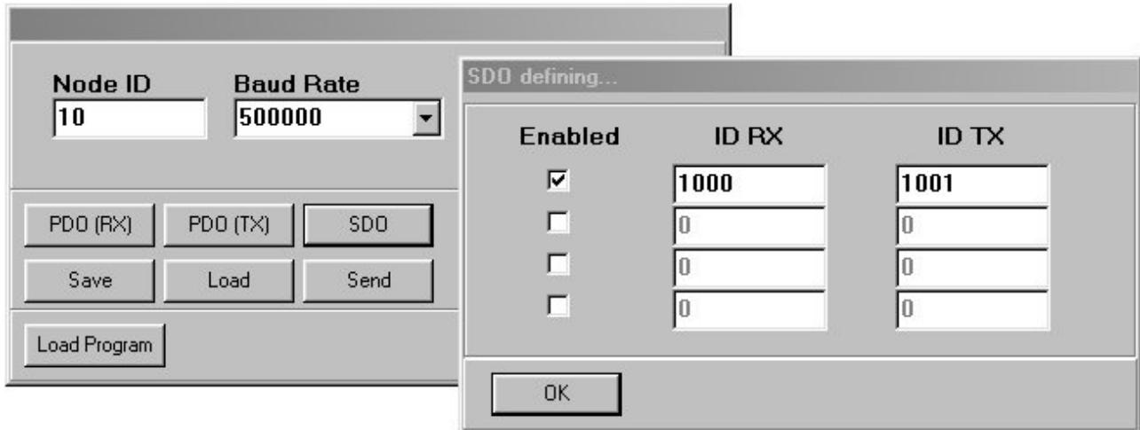
When the settings are complete, the configuration can be uploaded to the drive, clicking the “Send” button.
