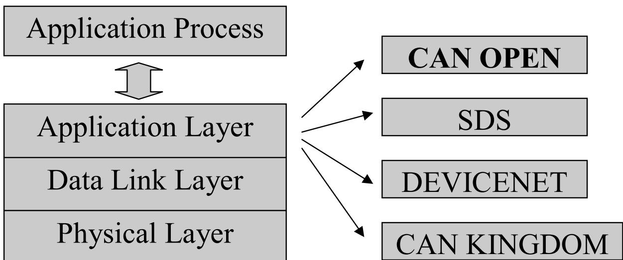
The Application layer interfaces itself with the different application processes e.g.: Drives, board of I/O etc... The Physical layer decides the physical transmission meaning, e.g. duplex twisted and shielded pair cable e/o, optical fiber and others, specifying its characteristics.
