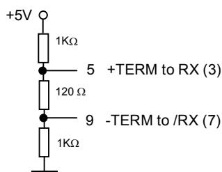
**The communication wires must be twisted and shielded.** The shield can be connected to the metal of the connector, because this part is connected to earth.
