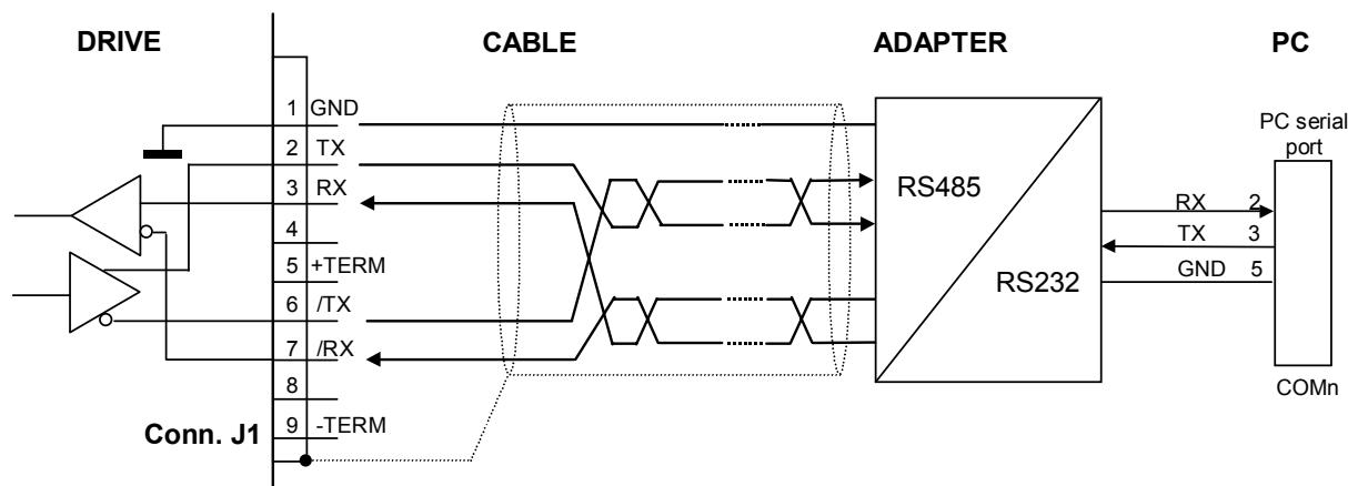
The serial line communicates in half duplex with four wires: RX+ and RX- are receiving wires for the drive while TX+ and TX- are the transmission wires. Connection can be made with only two wires connecting RX+ and TX+ and RX- and TX- on J1 connector.
