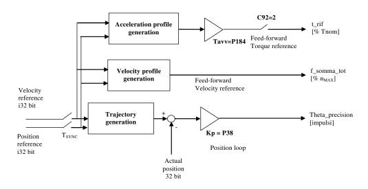
To have a good dynamic response, Kp=P31, Ta=P32 and Tf=P33 speed-regulator' gains and Kp=P38 regulator-position's proportional gain, must be adjusted.
