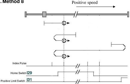
The initial homing speed is positive and equals to object Index=6099h Subindex=1 "Speed during search for switch". The home position is at the first index pulse (zero sensor) with the Home switch (**129**) at high level. The homing speed after Home switch rising edge is equal to object =6099h Subindex=2 "Speed during search for zero". If initially the Home switch is active the initial
