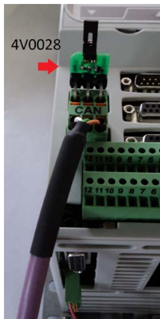
Fig. 13.1 (CAN bus termination with 4V0028)
