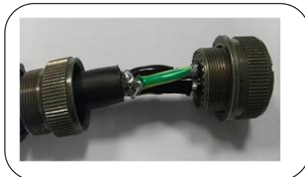
FIG. 23 (Drive side: example motor cable shield connection)
