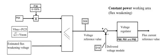
The flux current is normalized in relation to the magnetizing current (P73), the rotor flux is normalized in relation to the rated flux and is displayed as a percentage in d27. The stator voltage module is normalized in relation to the rated motor voltage (P62) and is displayed as a percentage in d18 and as a value in Volt rms in d17
