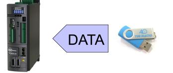
Parameters recipe can be loaded from the flash drive into the OPDE by using commands **S.02÷S.04**: the value setted will choose the recipe slot # to load from (choosing slot "0" will result in no operation). The difference between the commands is related to the kind of parameters loaded: S.02 loads both core and application parameters, S.03 loads only core parameters while S.04 loads only application parametes.
