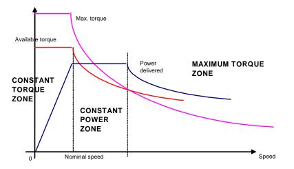
To ensure regulation stability, **P41** must be set with the Maximum torque divided by Rated motor torque. This limit will decrease during flux weakening with the square of the speed.
