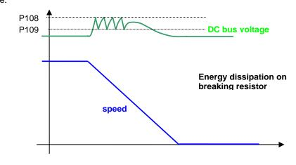
A maximum voltage limit allowed exists for the DC Bus voltage. This is checked by the software (threshold **P107**), and by the hardware circuitry: in case the voltage exceeds this level, the drive will immediately go into an over voltage alarm **A11** to protect the internal capacitors. In case of A11 alarm condition starts, verify the correct dimensioning of the braking resistor power.
