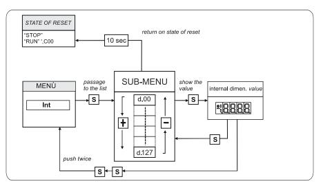
FIG. 16 (Visualization of the internal dimensions INT)
