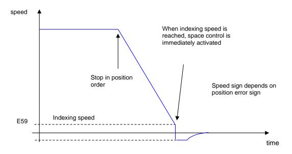
Anyway the speed reference generated by the position control can never exceed the indexing speed (in absolute value) set on E59.
