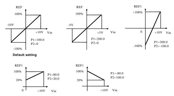
Note: for the offset parameters (P02, P04 and P06) an integer representation has been used on the basis of 16383, in order to obtain maximum possible resolution for their settings.
