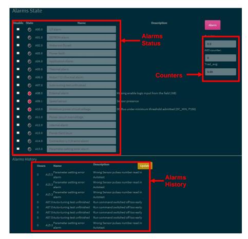
In the "Real time alarm state" are indicated the actual active alarms and, if they're present, the "Drive status" moves to "Alarm" and lights on in yellow. Every alarm has a description that help to know the cause of it.
