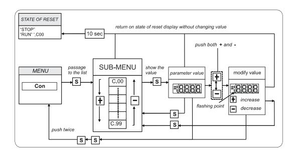
FIG. 15 (Submenu management connections CON)
