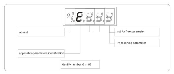
FIG. 3 (Application Parameters PAR)
