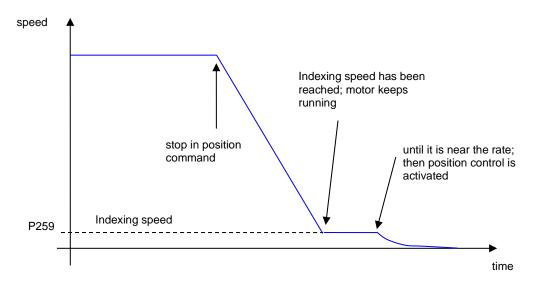
In this modality, to activate position control, it is necessary that the max. position error (180°) multiplied by the position loop gain (P38) being greater than the indexing speed (E59), thus:
