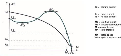
3-phase induction motor torque (M) and current (I) curve according to number of revolutions (N).
