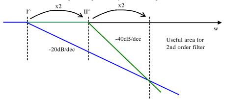
By taking as reference the 1st order filter time constant tolerated by the system, the 2<sup>nd</sup> order filter has to be set to double frequency (half time) so that it has the same phase margin.
