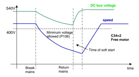
At the return of the mains, it will need to wait for the time of soft start for the gradual recharging of capacitors for the motor to be able to resume.
