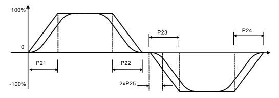
Rounding can be enabled on its own with C27=1, which will filter the overall speed reference value only.
