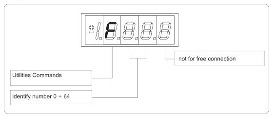
FIG. 10 (Fieldbus Parametrs FLB)
