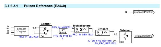
In this mode, the speed reference is given only in pulses ensuring maximum correspondence masterslave, but with a strong granular signal especially for low frequency input.
