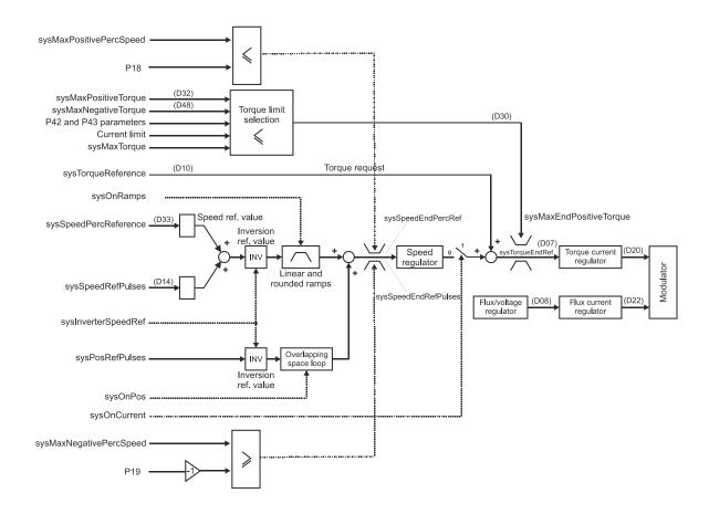
Regulation controls speed by default; here the application manages the speed reference values, and the torque request is used as a reference value added to the speed regulator output (feed-forward). Note that it is a torque control and not a current control, consequently during flux weakening the control automatically generates the request for the active current needed to obtain the required torque.
