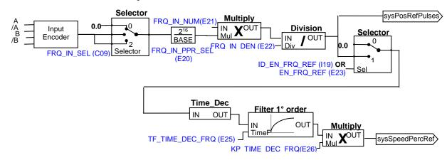
The frequency speed reference decoded in time ("sysSpeedPercReference") has to be enabled with **E23=1** o **I19=H**, it has very good resolution also for low frequency input, thus allows high speed regulator gains.
