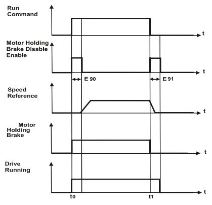
The figure shows the situation when the brake is disabled (on the left) and when is enabled (on the rigth). At time **t0** Run Command is given an internal timer is activated, at the same the digital output **032** goes to the high level.
