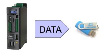
OPDE parameters are divided into 2 sets: "core" parameters and "application" parameters; "core" parameter are those contained into PAR, CON and FLB menues, while "application" parameters are those into APP menu ("base" application parameters from E00 up to E99 and "extended" application parameters from E100 up to E599).
