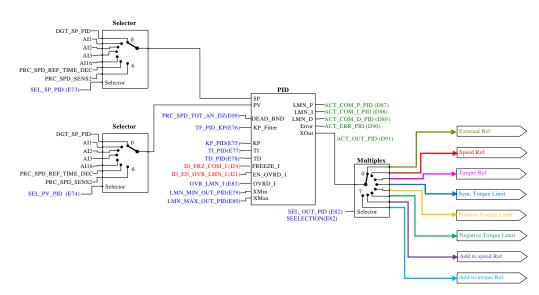
Below is shown the functional diagram of PID block.
