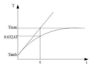
The picture above represent an hypothetical motor heating curve when loaded; it shows that  $\tau$  is the time in which the motor reaches the temperature **T=0.632\DeltaT+Tamb**, and  $\Delta$ T=Tmax-Tamb. In fact Tmax is reached about in  $5\tau$  (99.3% of  $\Delta$ T).
