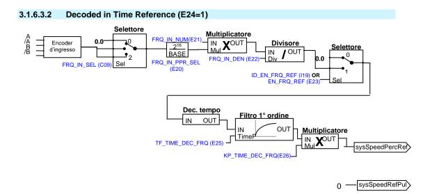
In this working mode the frequency speed reference is decoded in time with maximum linearity also for very low input frequencies.
