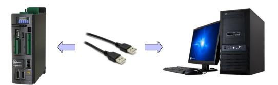
At the first connection the Operative System of the PC will ask for a driver that are powerd by BDF DIGITAL with the .inf file (that's good for both 32 and 64bit Windows OSes) and that can be downloaded by the website www.bdfdigital.it a the voice PRODUCTS/DOWNLOAD/UTILITY SW, folder DRIVER\_USB\_4T0008.zip.
