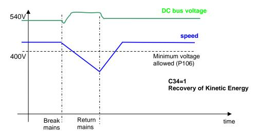
If the alarm condition starts, there is the possibility to enable, setting C35=1 the alarms to an automatic reset at the mains restore.
