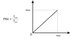
2. Characteristic FLUX WEAKENING AREA: When the maximum motor frequency is greater than nominal frequency automatically is set one characteristic point into nominal knee:
