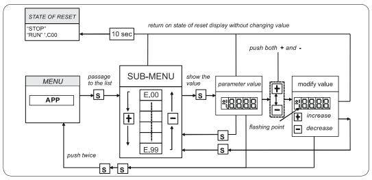
FIG. 14 (Submenu management application parameters APP)
