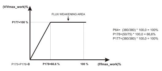
CURVE FOR MOTOR WORKING ALSO IN FLUX WEAKENING AREA
