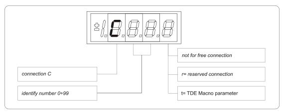
FIG. 4 (Connections CON)
